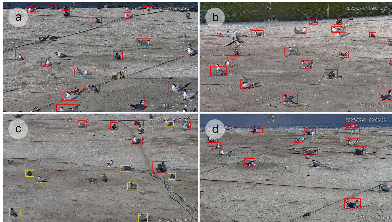
Fig. 5. Examples of the final algorithm performance using images from July 1, 2023 across different locations throughout the scanning of the island. Common Tern breeders in red squares and Little Tern breeders in yellow. (a) Identification of only Common Tern breeders, excluding standing individuals. (b) Identification of only Common Tern breeders, excluding other species breeders such as Black-winged Stilt (visible in the upper left corner). (c) Identification of both Little and Common Tern in close proximity, distinguishing between breeders and standing Little Terns. (d) Additional example of identification limited to only breeders terns despite close proximity to standing terns. (For interpretation of the references to colour in this figure legend, the reader is referred to the web version of this article.)
